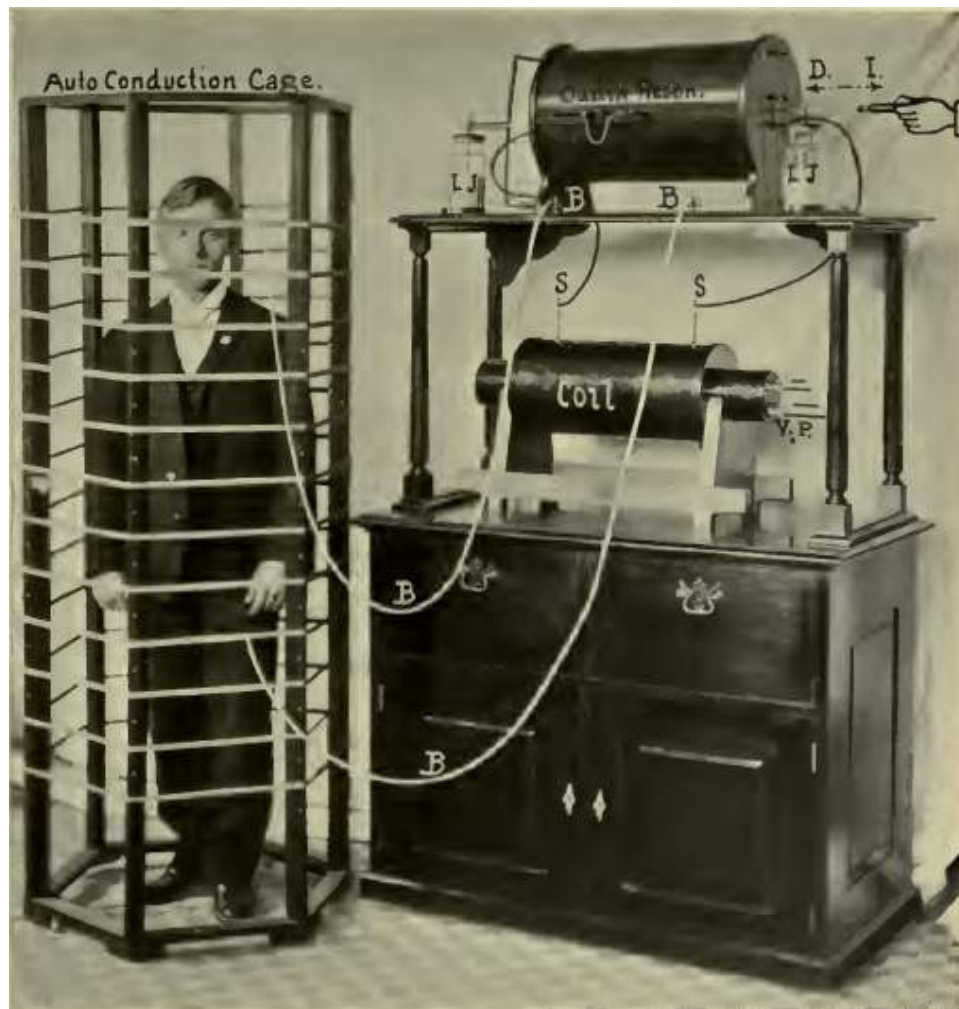
Figure 5 d'Arsonval's device for coupling currents to a body via a large, enclosing induction coil, called 'autoconduction.' [10]
